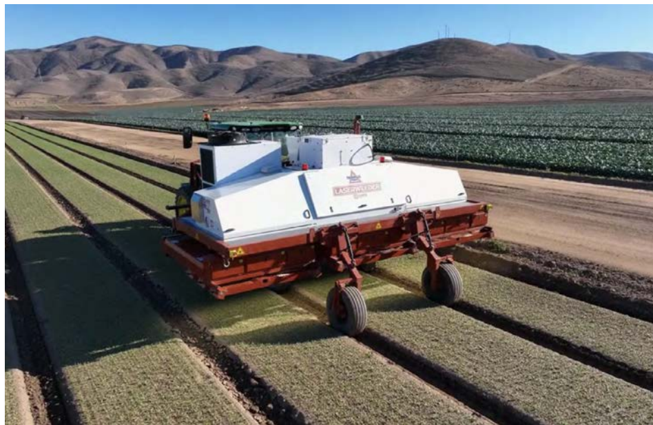
Corn & Soybean LaserWeeder in 40 and 60 foot configurations
