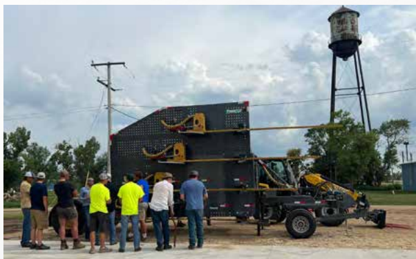
This fiber-cutter is a unique piece of hydraulically driven pull-behind sickle mower that can cut hemp with 1, 2, 3, or 4 blades simultaneously at varying heights.
